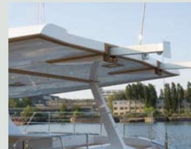
in welded light and strong Alcan Marine Sealium 5383 marine grade aluminium alloy commenced in February 2008. By August last year her twin hull assembly (which was constructed upside down like all Sunreef's custom one-design yachts) had been turned over and the upper deck and flybridge lowered onto it.
