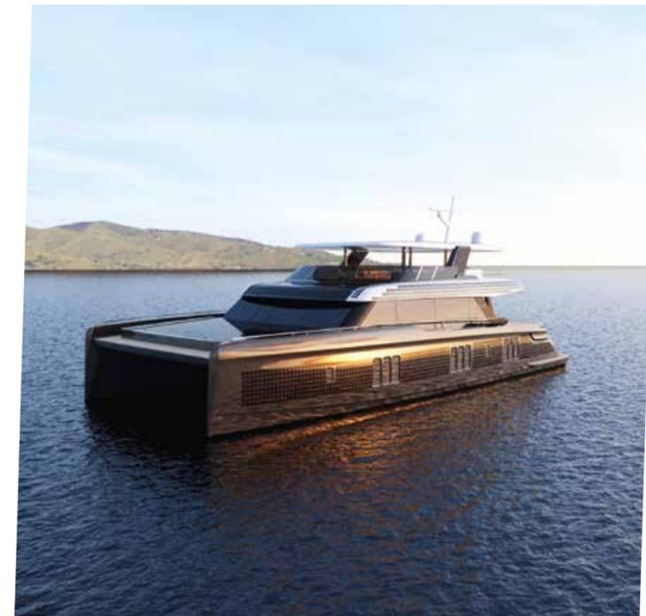
First up: Solar Skin. Sounding like the sea-hardened hands of an old skipper, Sunreef's Solar Skin are solar panels that have been cleverly and subtly integrated into the yacht's framework. In fact, they can be mounted pretty much anywhere including on the hull, superstructure and mast. They are the industry's lightest panels. Which, if you're in the business, know is a big deal.
